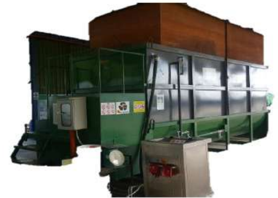
ANAEROBIC DIGESTOR (100kg) Located in Port Dickson, Hang Tuah Jaya, Kulim Hi Tech and Pulau Tuba (Langkawi)
