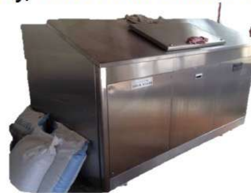
COMPOSTING MACHINE (500kg) Located in Fraser Hill (tourist attraction) to treat food waste on daily basis
